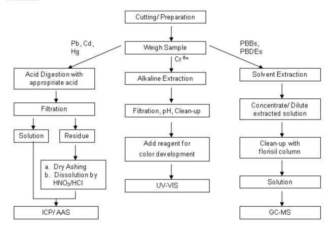
Note: 1) Boiling water test method was also performed for the analysis of Cr (VI) in metal sample.
